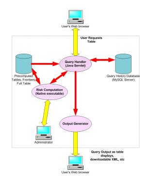
Figure 2: Table server prototype: System architecture. Output formats include screen display and XML.
