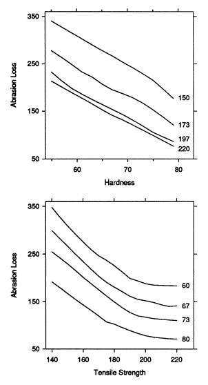
Figure 11. Abrasion-Loss Data. Conditioning plots show a loess fit to the abrasion-loss data, with f=.5. The graphs suggest the dependence on hardness is linear and that there is no interaction between tensile strength and hardness.
