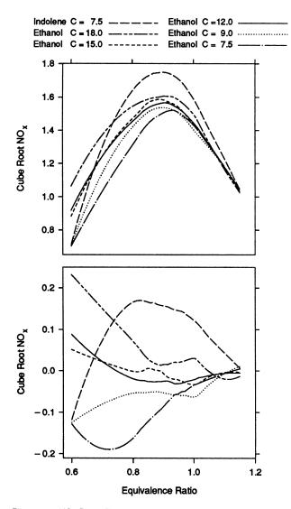
Figure 15.  $NO_x$  Data. The top panel shows the six separate smoothings of  $NO_x$  as a function of equivalence ratio. The bottom panel shows the curves with a mean curve subtracted. The graphs show a strong interaction among the independent variables that cannot be removed by a nontrivial transformation of the dependent variable. Thus an additive fit is not possible for these data.
