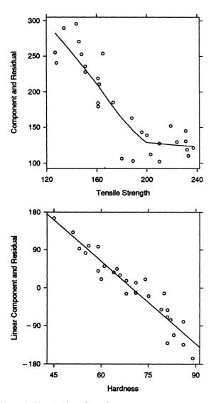
Figure 13. Abrasion-Loss Data. Component-residual plots show the additive fit to the abrasion-loss data, with f=.75. The curve on each plot is the estimated component function for one independent variable, and the plotting symbols show the component function value plus the residual for each observation.
