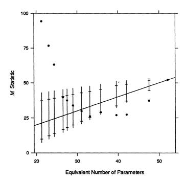
Figure 14.  $NO_x$  Data. The data are from an experiment studying the dependence of  $NO_x$  exhaust emissions on equivalence ratio, compression ratio, and type of fuel. The figure is an M plot for locally quadratic fitting, with f ranging from .4 to 1 in steps of .05. The type of fuel and the level of compression ratio, which took on one of five values, were both entered as categorical variables. On the basis of the plot, f was chosen to be .85.
