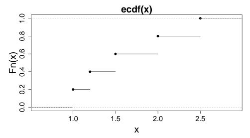
There are 5 jumps, each located at the position of an observation. Moreover, the height of each jump is the same:  $\frac{1}{5}$ .
