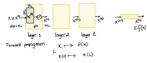
The construction can be generalized recursively to arbitrary numbers of layers. Each layer is a linear combination of the outputs from a previous layer (a multivariate operation), followed by a non-linear transformation via the logistic function  $\phi$ . Let  $x \equiv x^{(0)}, y \equiv x^{(L)}, n_0 = n, n_L = 1$  and define the recursion:
