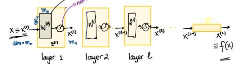
The construction can be generalized recursively to arbitrary numbers of layers. Each layer is a linear combination of the outputs from a previous layer (a multivariate operation), followed by a non-linear transformation via the logistic function  $\phi$ . Let  $x \equiv x^{(0)}, y \equiv x^{(L)}, n_0 = n, n_L = 1$  and define the recursion:
