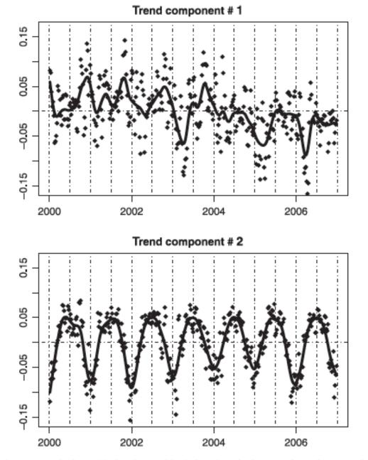
Fig. 4. Smoothed empirical orthogonal basis functions for log-transformed two-week average concentrations of PM2.5 in the Los Angeles area. The first smoothed component explains 27.5% of the variation in the matrix of log-transformed 2-week average PM2.5 concentrations while the second component explains only 9.4% of the variation.
