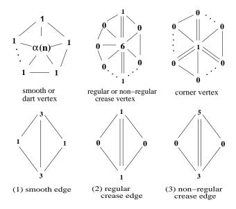
Figure 3: Vertex and edge subdivision masks. Double lines denote sharp edges.
