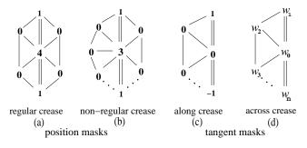
Figure 4: Position and tangent masks for crease vertices.
