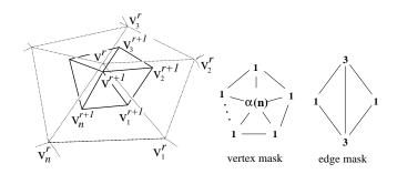
Figure 1: The neighborhood around a vertex  $\mathbf{v}^r$  of valence n (left); Loop's vertex mask (center); Loop's edge mask (right).
