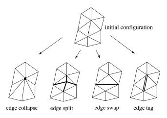
Figure 5: Elementary mesh transformations.
